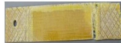
Fig 10.2 Chapsten E-Glass Epoxy Specimen after Tensile Test
