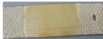
Fig. 10 Tensile Test Specimens of Glass Fiber Epoxy, Chapsten E-Glass Epoxy and Glass Fiber Polyester Epoxy
