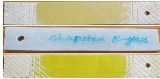
Fig. 10 Tensile Test Specimens of Glass Fiber Epoxy, Chapsten E-Glass Epoxy and Glass Fiber Polyester Epoxy
